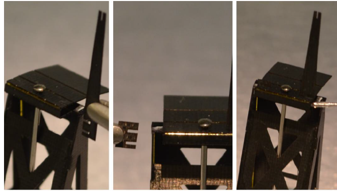
Figure 3.26: Glue E-Clips in Place [28].
