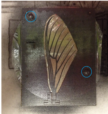
Figure 3.17: Wing Card Aligned on PLU For Cutout.
