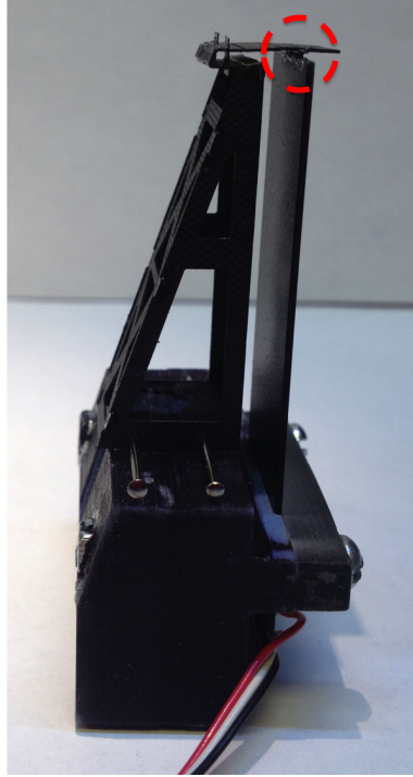
Figure 3.30: PZT Attachment to Base.
